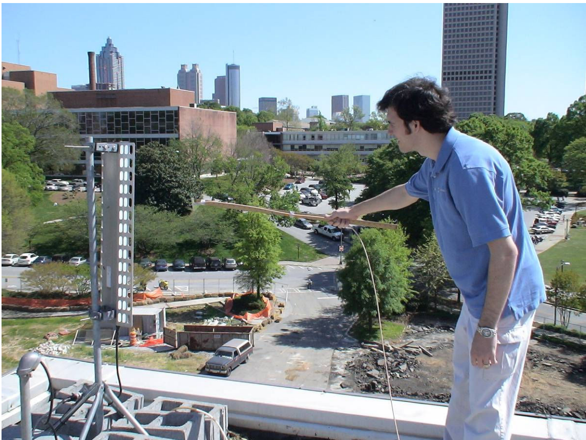
Figure 11: One-meter test measurement process to verify estimates of the transmitter output power of the Van Leer AP.
