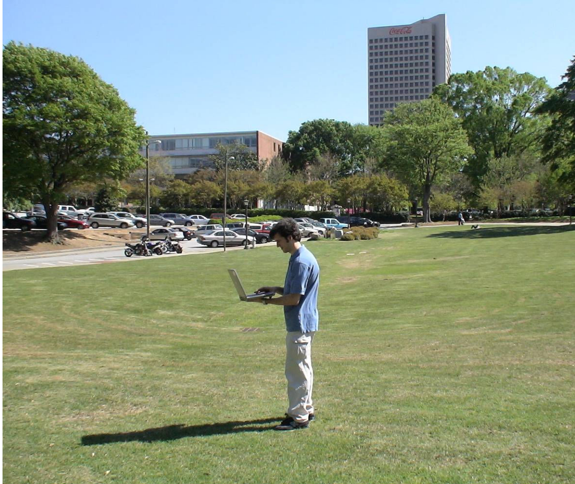
Figure 2: When taking measurements, the laptop was kept in the orientation shown, with the top of the WLAN card pointed toward the zenith sky. This was done to maintain received pattern consistency throughout the survey.
