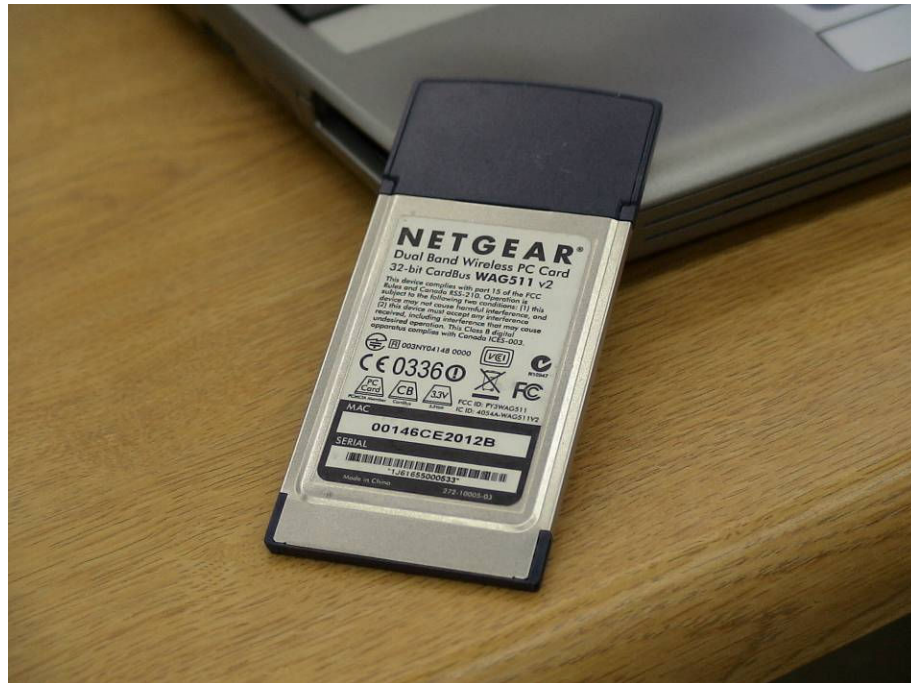
Figure 1: The NETGEAR™ WLAN card used as the receiver device in all surveys
