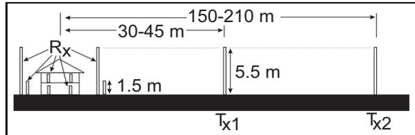
Fig. 1. Transmitters (TX) and receivers (RX) at different heights and separation distances.
