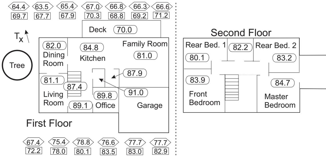
Fig. 2. Summary of 5.85 GHz path loss measurements at the Rappaport home.
