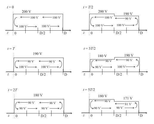
(a) Each step-down in voltage occurs during even multiples of a transit time:
