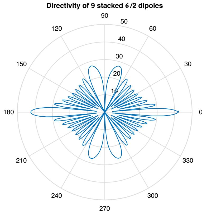
Half-wave dipole array of 9 element(s)
