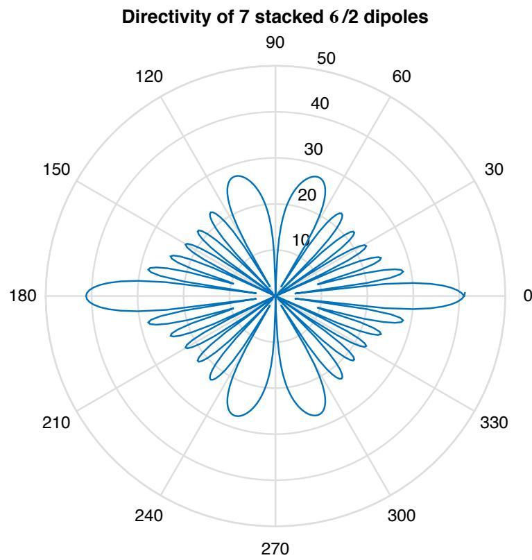
Half-wave dipole array of 7 element(s)
