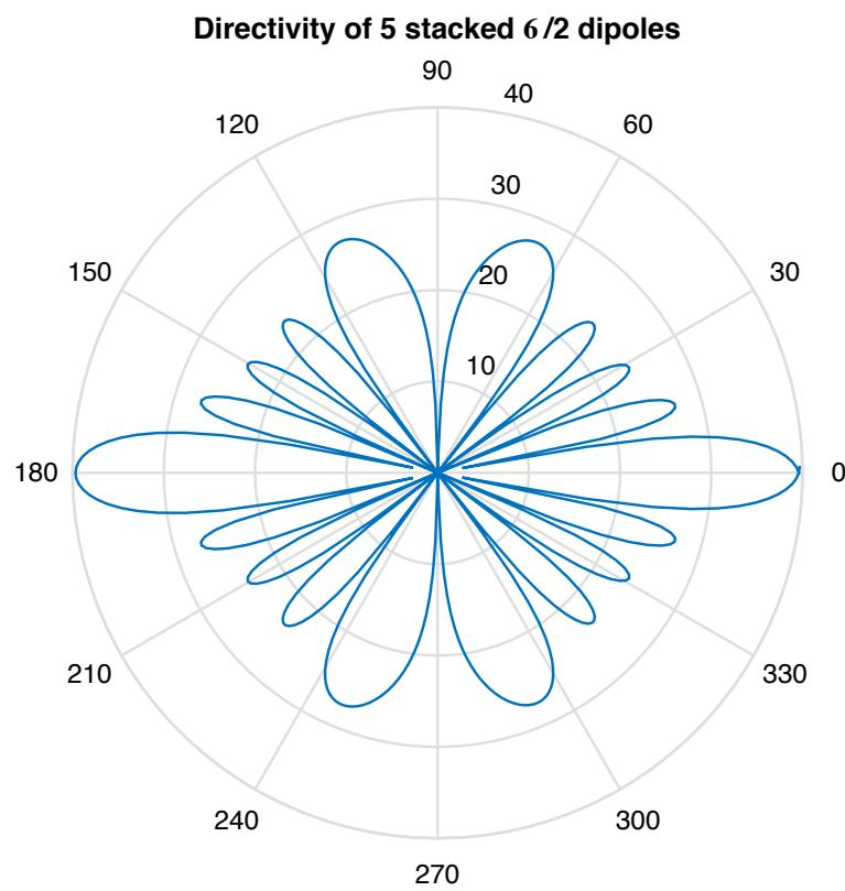
Half-wave dipole array of 5 element(s)
