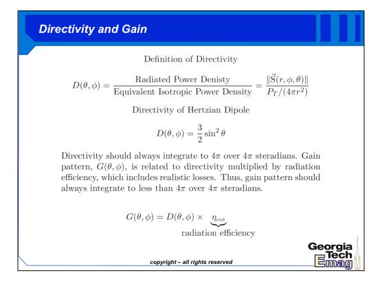
Another quantity that we can calculate from the Hertzian dipole fields is the directivity. Directivity is defined as the ratio of power density radiated in a particular direction to the average power density radiated in the system. Under this definition, directivity will always integrate to 1 over the full 4pi steradians of space. An example calculation for our Hertzian dipole is shown above.
