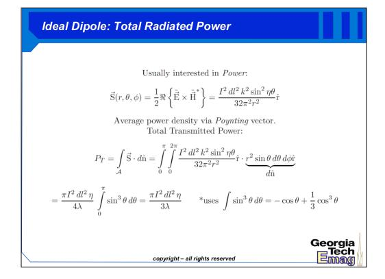
Let's calculate the total amount of power radiated by the Hertzian Dipole. To do this, we calculate the Poynting vector (units of  $W/m^2$ ) from E and H. Then we integrate this quantity around 4pi steredians. This gives us total power as a function of current magnitude, I (Amps), wavelength, and infinitesimal length Delta l. Note how the Poynting vector is always pointing away from the origin, regardless of point of observation.
