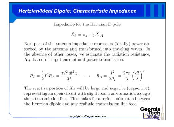
We can estimate the impedance of a very short dipole at the end of a transmission line by using this result from the Hertzian dipole. Say we take a tiny dl-length of line and bend it back. We know that this load would appear highly capacitive and can calculate the result from the Smith chart or the load transformation formula.
