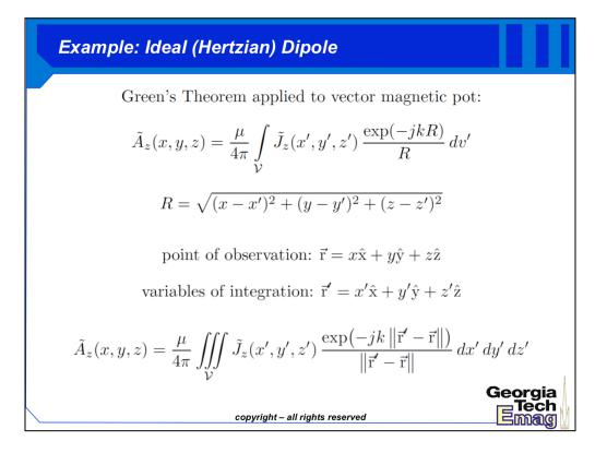
This simple solution for Az given a possible source at the origin can be used to synthesize a field from any z-directed spatial distribution of current. Thus, plug any given Jz into the equation above and solve for Az. Recall that the standard quantities of electromagnetics – E-field, H-field, and Power – may all be derived from Az after this integration is complete.
