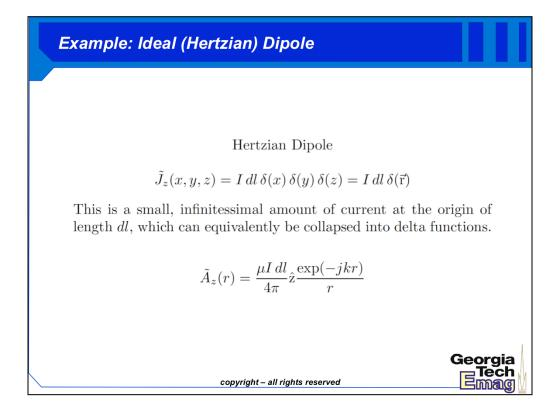
The simplest radiating system is the Hertzian dipole, resulting from an infinitesimal current element at the origin flowing in the z-direction. This can be described mathematically as a Jz with three delta functions w.r.t. x, y, and z. Plugging this into our formula, we get the above expression for Az.
