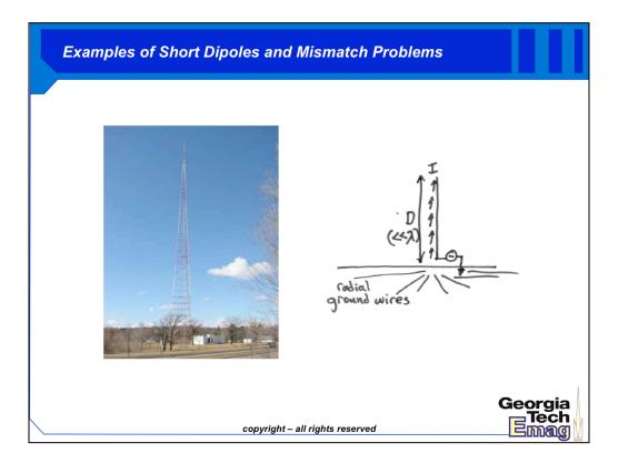
One example of a short dipole is the AM radio transmit tower. AM radio waves have very long wavelengths (> 300m), so that even the tallest towers can only support radiating wires that are a fraction of this length. In many cases, the radiator behaves effectively like a short dipole with large capacitive mismatches.
