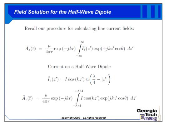
So let's simplify this expression for a case of current distribution I(z) that exists only on the z-axis. This corresponds to the case of a wire antenna, which is one of the most common instances in basic antennas. The most common of these common antennas is the half-wave dipole (HWDP), because it is a compact, efficient radiator with many different implementations in practice. It may be used by itself or as the radiative element in a reflector (dish) based antenna.
