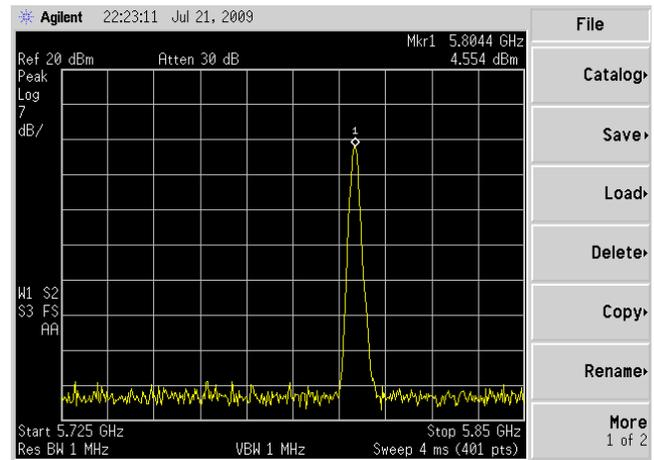
**Figure 26: Frequency hopping is functional and no side band signal is observed within required band.**
