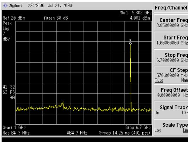
**Figure 25: Received signal over 1-6.7 GHz band on spectrum analyzer.**
