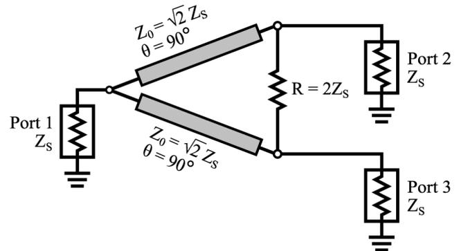
**Figure 6** The design for a basic equal-split power divider.  $Z_s$  in this case is 50  $\Omega$ . Figure from [4].
