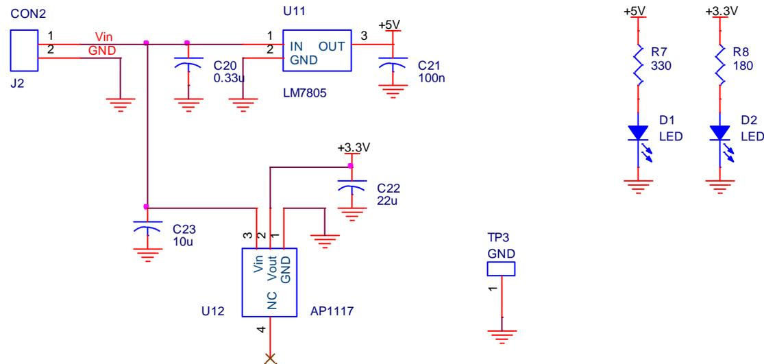
Figure 28: Schematic of power management
