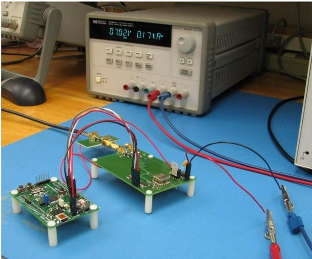
**Figure 24: The system was powered by 7 voltage power supply and connected to spectrum analyzer for compliance test.**
