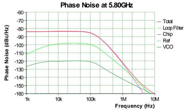
Figure 4: Simulated phase noise performance of designed PLL system.
