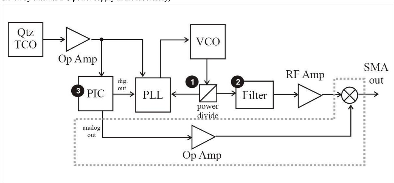
Figure 1: System Block Diagram of a 5.8 GHz RF Signal Generator
