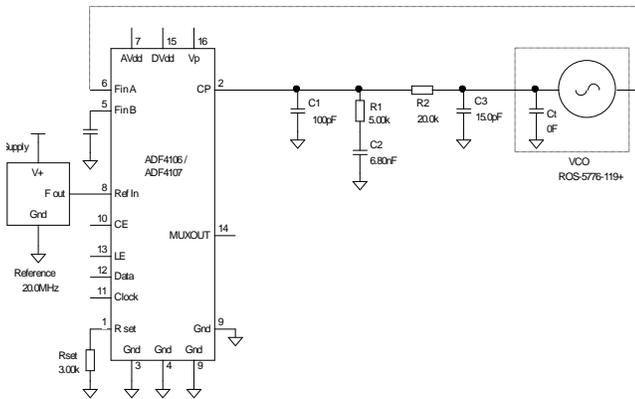
Figure 2: Schematic of loop filter.
