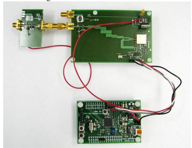
Figure 23: Populated signal generator board connected with PIC evaluation board.
