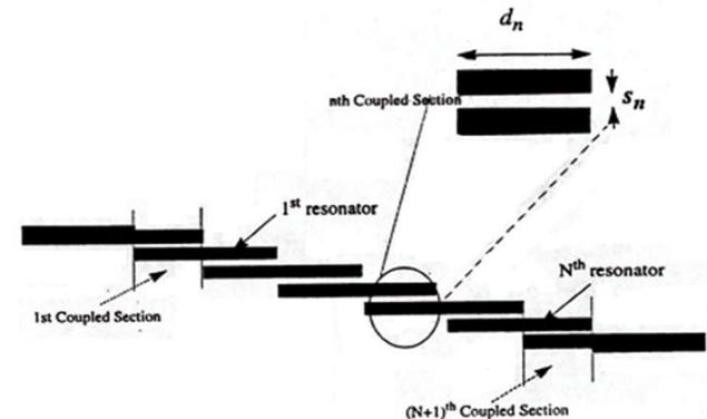
Figure 14: Parallel Coupled Bandpass Filter
