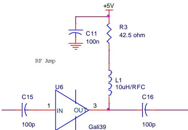
Figure 21: Schematic of one stage RF amplifier
