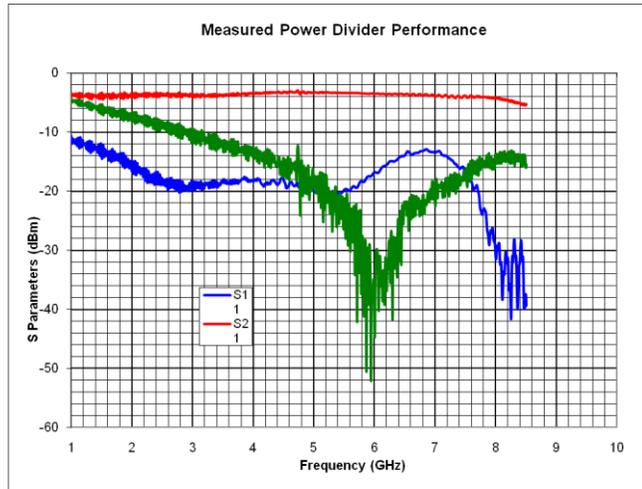
Figure 13: The measured performance of the power divider.
