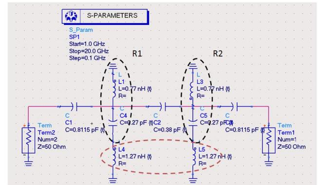
Figure 15: Schematic of alternate Filter
