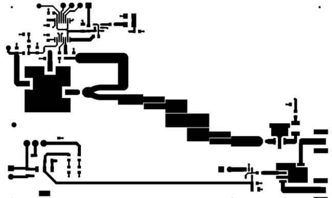
Figure 22: Top layer PCB layout of signal generator
