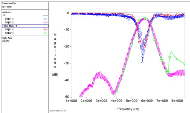
Figure 20: Correlation of Measurement and Simulation
