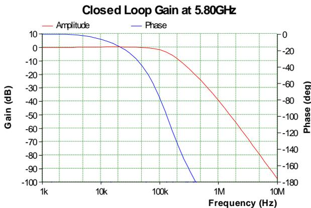
Figure 3: Gain and Phase Margin
