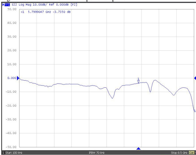
Figure 11. Measured S22 of the power amplifier
