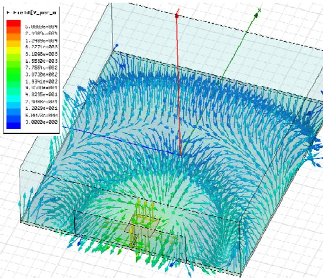
Fig. 7. This figure shows good electric field patterns of close to 6kV/m from the patch antenna.
