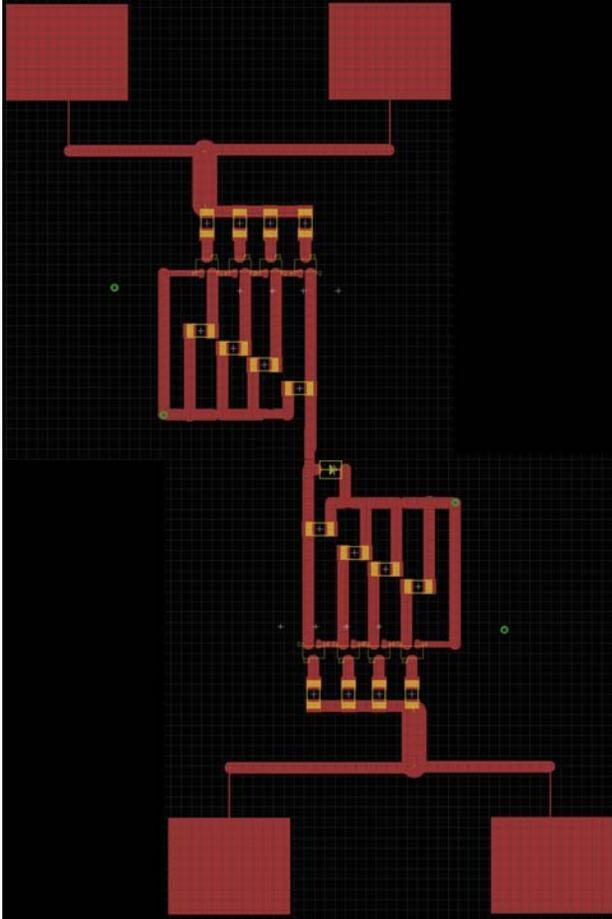
Fig. 4. Charge pump layout with patch antennas.
