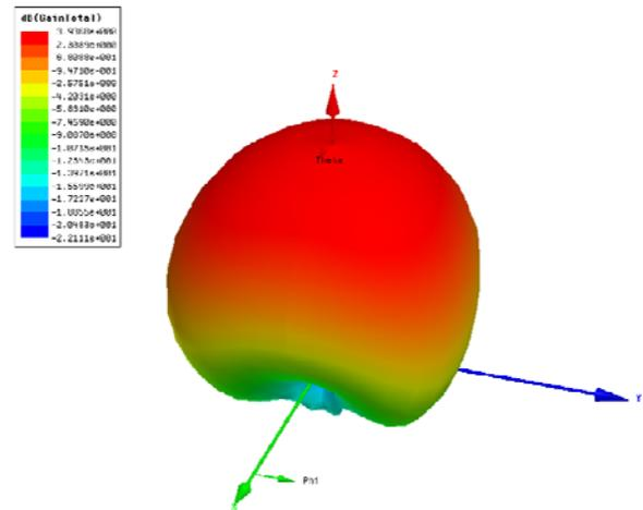
Fig. 6. Radiation gain pattern as simulated in HFSS.
