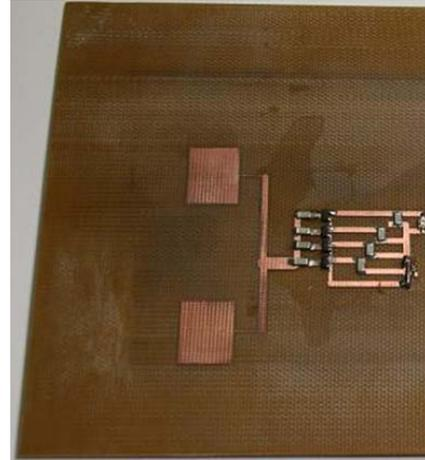
Fig. 10. Fabricated charge pump circuit.
