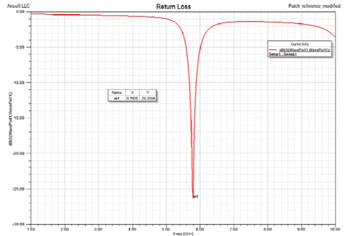
Fig. 5. Simulated return loss shows that the antenna is well matched at the desired frequency of 5.8 GHz.
