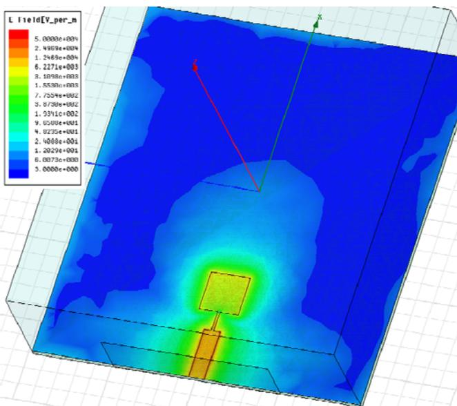
Fig. 8. The magnetic current is fed uniformly into the patch through the quarter wave transformer.
