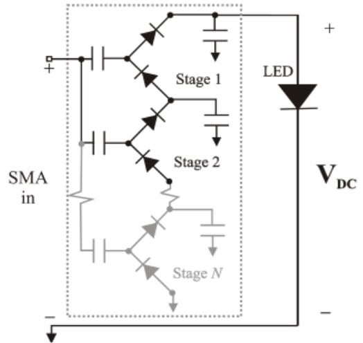
Fig. 1. General circuit diagram of an N-stage Dickson charge collector loaded with an LED.
