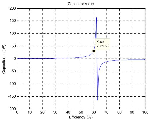
Fig. 2. Capacitance plotted versus efficiency to determine optimum capacitor value.
