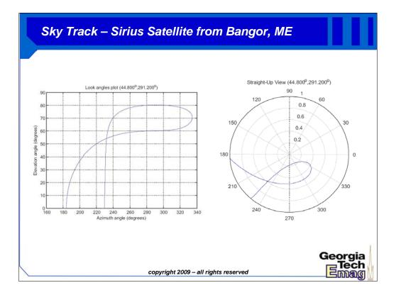
Here is a sky track for Bangor, Maine, which is obviously a lot farther north than Atlanta (44.8 degrees latitude). Notice how well the satellite in Tundra orbit still stays above the 45-degree elevation line in its sky track. By now, however, the geostationary satellites would have dropped fairly low to the horizon. Their signals would be easy to degrade with foliage or terrain obstruction. Stephen King probably subscribed to Sirius satellite radio instead of XM radio when it first came.
