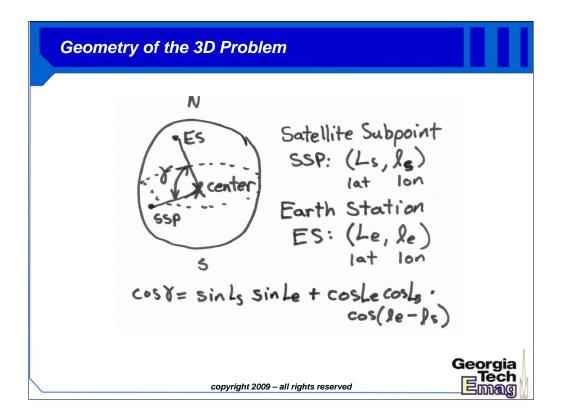
To translate this into 3D, we must first calculate this angular distance gamma from two pairs of longitude and latitude, one for the SSP and one for the ES. Given the geometry above, we need to define several helper variables (psi, beta, and little delta) based on the earth station position (Le, le) and the SSP (Ls,ls). Uppercase L refers to latitude and lowercase l refers to longitude in the system of equations above.
