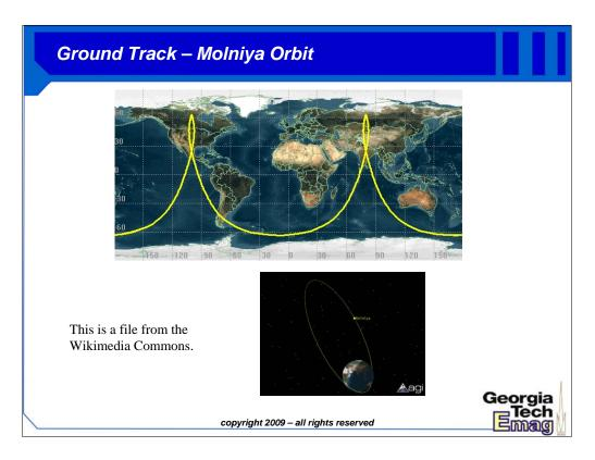
Although we discussed elliptical orbits, we didn't necessarily talk about applications that require elliptical orbits – most of our discussions of real satellites have centered on circular orbits. Here is one example of an eccentric orbit called a Molniya orbit.
