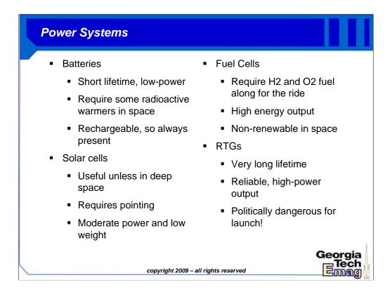
**Batteries**: They have stored energy, which is utilized by the spacecraft when required. Although this technology is well understood, reliable and consistent; it is just not powerful enough to meet the needs of a space mission. However, batteries can be used to store the energy created by some other means. Hence, batteries can be used for storing excess power on the relay satellite and for powering the three probes during their descent into Neptune.
