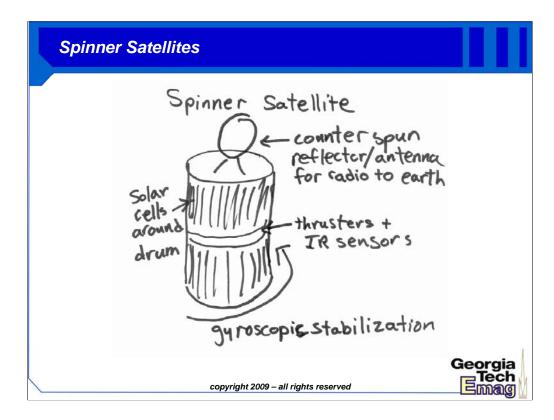
A "spinner" satellite is spun into orbit so that its gyroscopic forces keep the satellite from twisting into an undesired orientation. A communications antenna is typically "de-spun" so that it points towards earth even though the satellite is spinning. Sensors along the drum of the satellite use IR probing to makes sure the satellite antenna points to earth. Small thrusters along the drum can perform timed-fires for orbital control.
