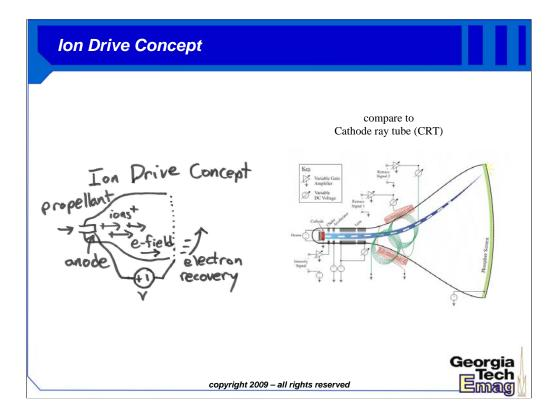
Once in space, other forms of propulsion become feasible. For example, an ion drive may be used to propel spacecraft to higher earth orbits or onto deeper space missions. Such a drive works by ionizing gasses and electrically accelerating them out the back side of the drive. Again, conservation of momentum leads to thrust in the forward direction.
