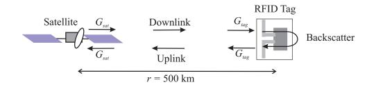
(a) For a passive tag, at least  $20\mu$ W must be received by the tag from the satellite interrogator in order for the tag to power-up. How much transmit power must be sent by the interrogating satellite to make this happen? Based on your knowledge of spacecraft power systems, does this seem reasonable? (**15 points**)
