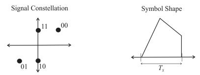
(a) In the two graphs below, make a rough sketch of the in-phase and quadrature signals that would be sent into the alien's IQ-modulator for the following data sequence: 00100111 (left-to-right is earliest to last bit) (15 points)
