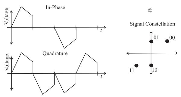
(b) This signal has sharp transitions, which makes for inefficient spectral use.
