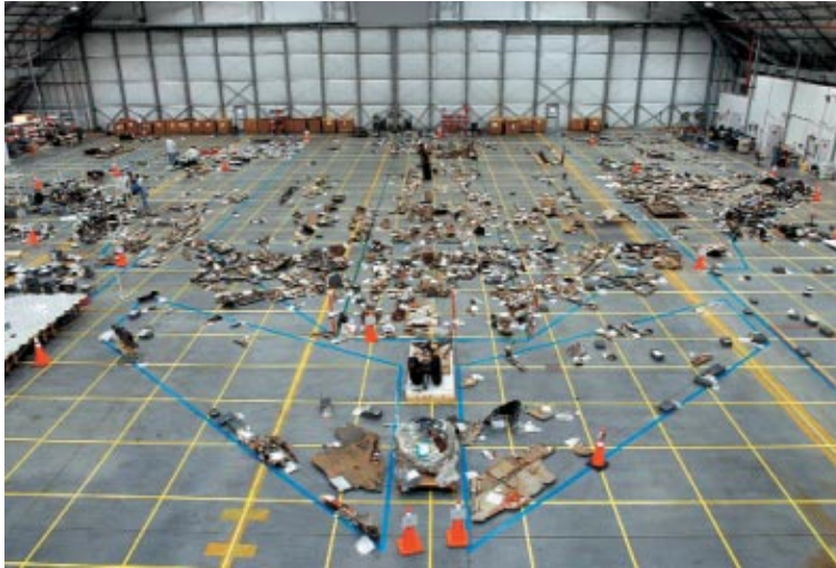
More than 80,000 pieces of debris—roughly 40 percent of the shuttle's mass—were recovered from the Columbia. Here, they are placed within an outline of the shuttle, indicating where they were on the vehicle before breakup.
