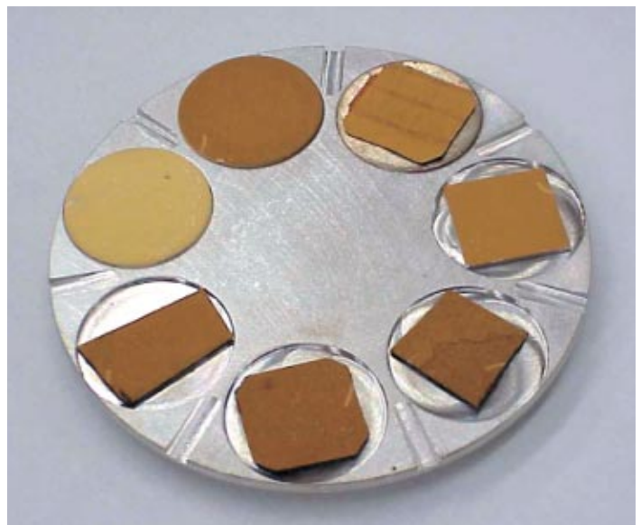
right. After a simulated 10-year exposure in geosynchronous orbit, the paints turned brown, as shown in the photo on the right.
