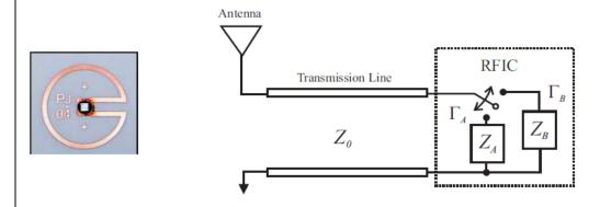
When the RFID tag is placed on a metal surface, the topology of the circuit changes dramatically. One way to model this new topology is with a *microstrip* transmission line; the antenna and feed traces now beat against the metal surface as if it were a ground plane underneath the plastic/dielectric, just like a printed circuit board!
