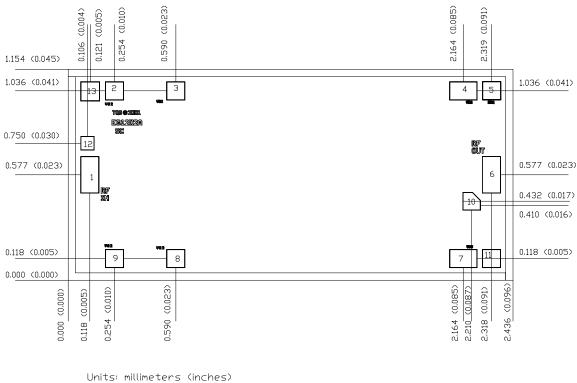
Units: millimeters (inches) Thickness: 0.100 (0.004) Chip edge to bond pad dimensions are shown to center of bond pad Chip size tolerance: +/- 0.051 (0.002)
