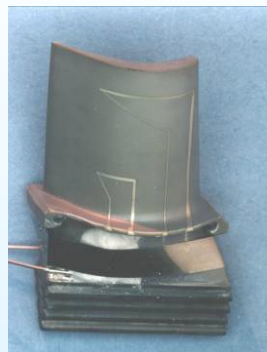
Pt- Pt/Rh temperature sensor to T=1200^{\circ}\text{C}
