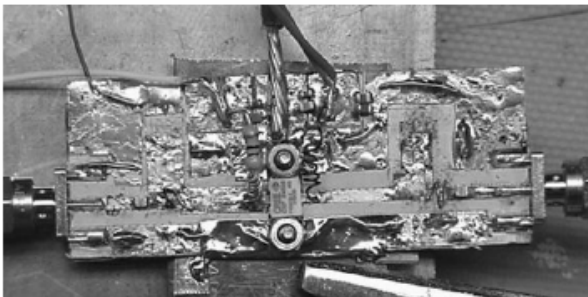
High Temperature SiC RF Amplifier Prototype (Softronics)
