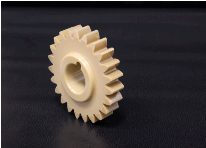
Ceramic gear with potential for operating at Venus operating temperature
