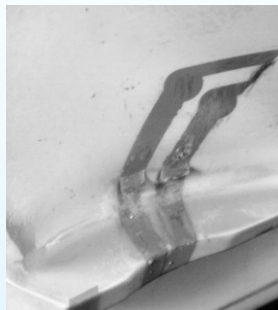
PdCr strain sensor On Alloy to T=1000^{\circ}\text{C}
