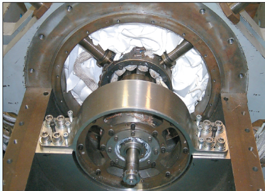
Switched-Reluctance Motor: 8,000 rpm at 540°C (NASA GRC)
